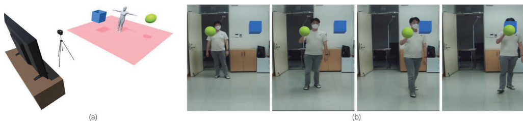
Figure 27. AR interaction: (a) The user can see the virtual objects on the screen. (b) The virtual objects appear located away. Walking close to the ball, the user picks it up. Walking toward the box, the user hits the box with the ball.
