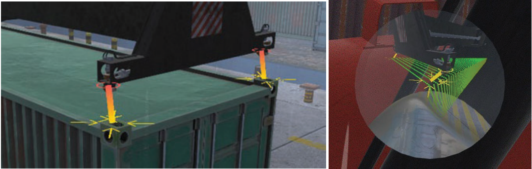
Figure D. 7. When the user has to lock a container, color-coded AR lines appear to indicate the proper alignment between twist locks and corner castings (on the left). Another experimental feature is a real-time LiDAR scan of the container that shows a 3D rotatable
