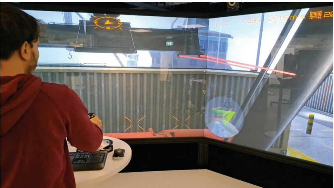
Figure D. 8. The user aligns the spreader's twist locks to the container's corner castings by controlling the joystick.
