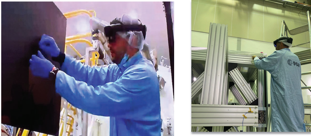
Figure 10. VirWAIT use cases. Left: Thermocouples installation to SMILE. Right: Sensors installation to TEDY.
