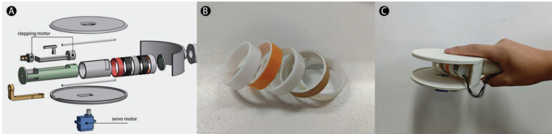
Figure P. 2. (A) Our device uses a two degree of freedom cylinder as the base, with some material rings sliding on it to present various tactile sensations. (B) Material rings are interchangeable and can be customized to render any texture. (C) The user is using a material tactile display.
