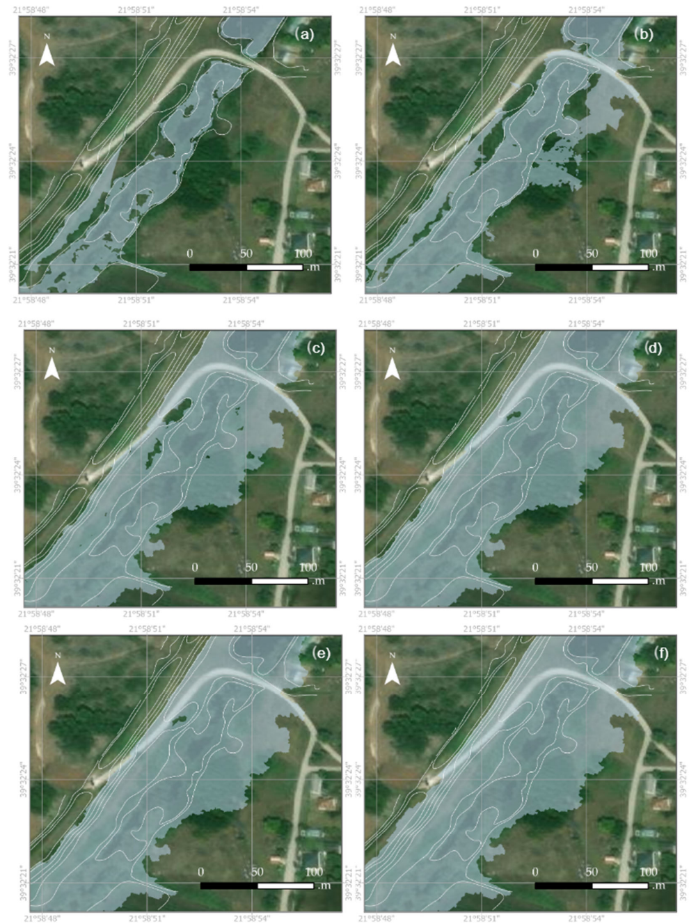
Figure 7. Two-dimensional visualization of the flood scenarios at (a) 1 m, (b) 2 m, (c) 3 m, (d) 4 m, (e) 5 m, and (f) 6 m of flood height.
