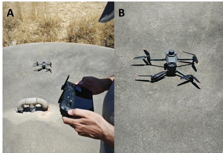
Figure 9. A) Drone pilot operating the UAV during take-off near the survey site; B) Close-up of the DJI Mavic 3 drone on the ground before flight.
