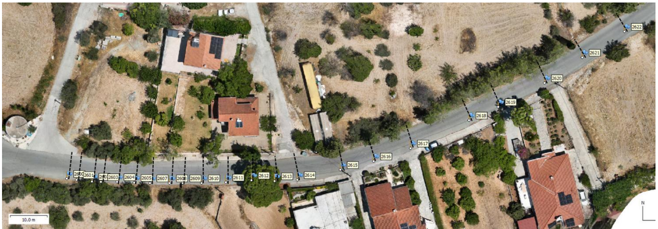
Figure 8. Survey map of GPR measurements in Doros village. Black lines indicate the locations where the GPR profiles were acquired during the field campaign (vertical towards the road) (Drone image captured on 04 July 2025).
