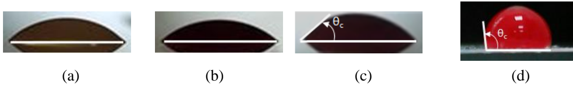
Figure 3.7. Images of drops on the glass surface. (a): From the Newtonian fluid, (b): From the non-aggregating blood and (c): From the whole blood. \theta_c is the measured static contact angle. In panel (d): Representative image of whole blood drop on the adhesive tape.
