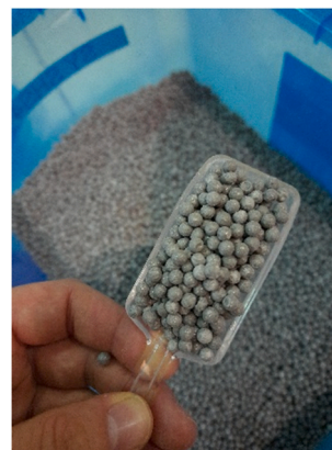
Fig. 1. Pre-coated steel foam hollow spheres are used for specimen creation.
