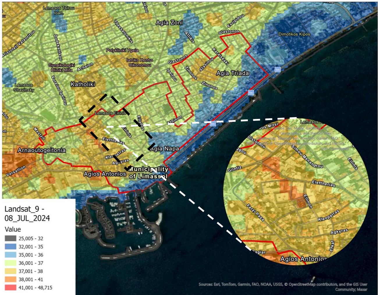
Figure 6 Thermal satellite image from LandSat-9 in Limassol with spatial resolution 30m x 30m acquired on 8th of July 2024 at 08:20 a.m.
