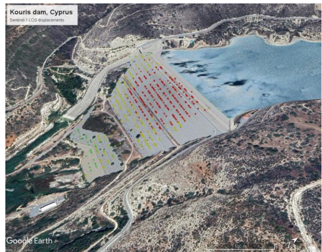
Figure 3. 3D view of Sentinel-1 line of sight displacements in Kouris dam from 2015 to 2023.
