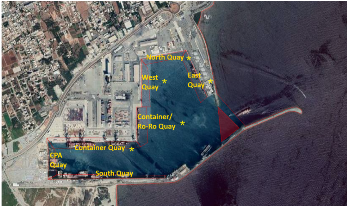
Figure 12: A satellite view of the Port of Limassol, Cyprus illustrating its seven berthing quays (taken from [7]). Note: * with quays indicates that these are used for commercial purposes only.
