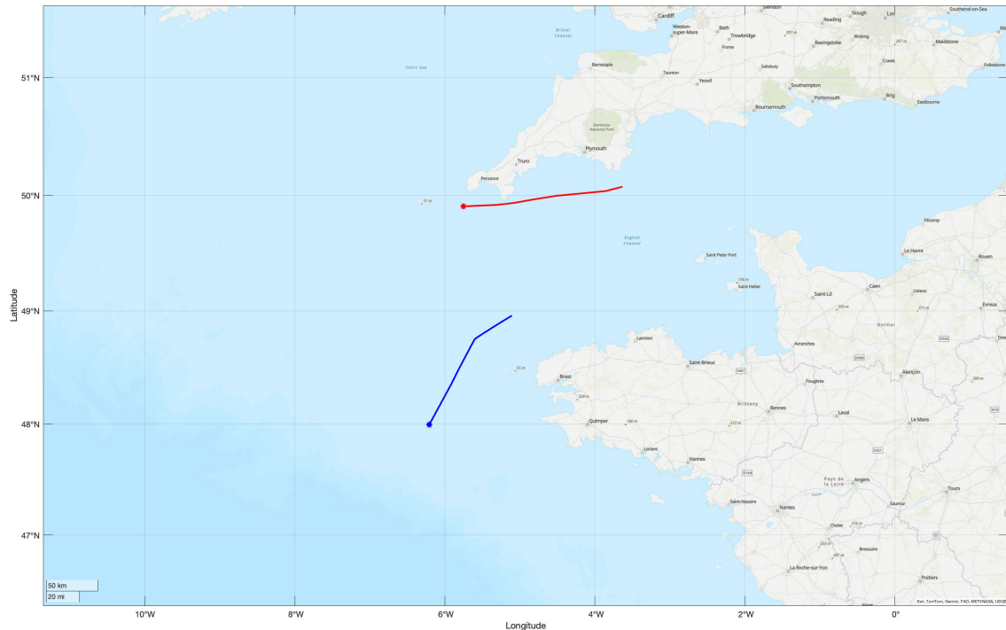
FIGURE 6. Example featuring real trajectories (duration 1 hour, sampling time T = 9.8467 s). The ownship is shown with a blue line and its start point is denoted by an asterisk. The motion of the target ship is shown in red and the initial point is shown with a circle. Latitude–longitude coordinates (degrees) are shown directly in the plots; the 50 km scale bar provides a visual distance reference.
