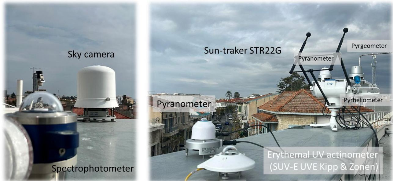
Figure 1. Limassol Solar Radiation Station. The two platforms, one with the spectrophotometer and and All-Sky Camera and the other one with the Sun-tracker, pyranometers, pyrgeometer, pyrliometer and one erythemal UV actinometer
