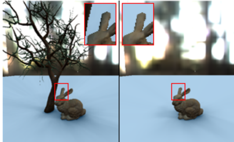
Figure 27: An object (bunny) may act as both occluder and receiver. The bunny as a receiver (left) has shadows cast on it, in contrast to the bunny (right) which act only as an occluder.
