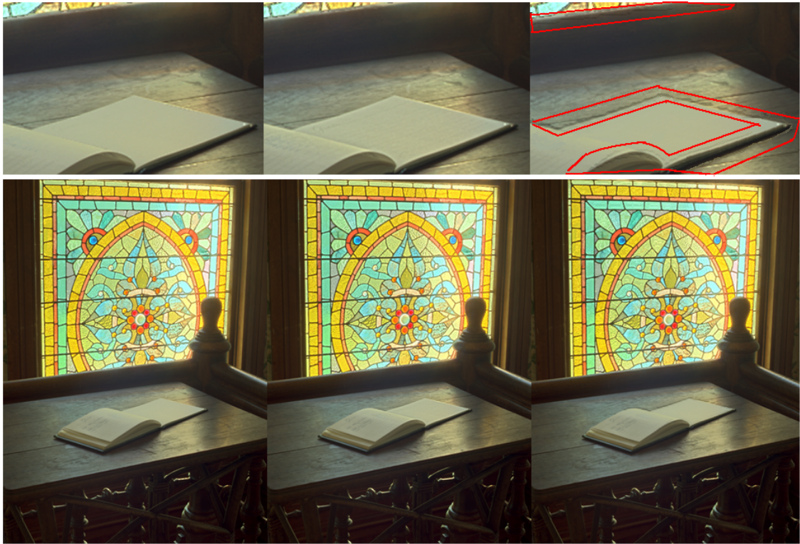
Figure 32: Tonemapped results of Desk image; close-up at the book area (top) and full resolution image (bottom). Results are given for selective tonemapping using sobel filter (left), local tonemapping (middle), selective tonemapping using saliency map (right). Artifacts in the transition areas between dark and bright regions, are strongly visible in the output obtained when saliency map is used (red marked areas).
