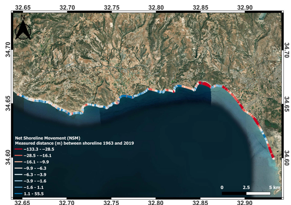
Figure A1. NSM in the study area. The more red the coastline, the more erosion it has undergone, while the bluer it is, the more deposition it has seen.
