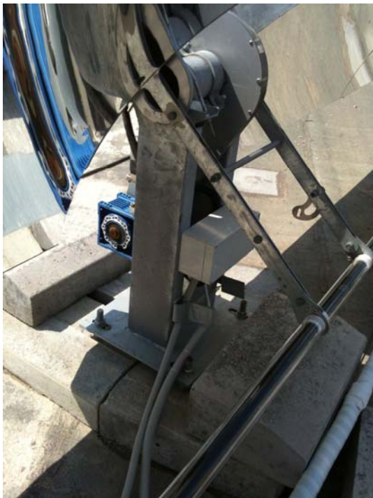
Fig. 3 Photo of the motor of the tracking system and central support of the collector (at park position).
