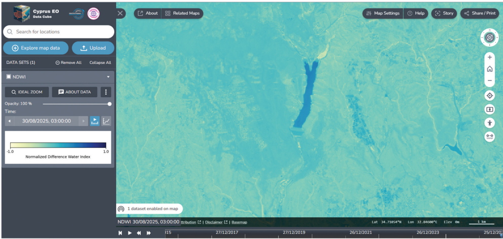
Figure 8. Cyprus Earth Observation Data Cube browser. Example screenshot from the visualization platform illustrating a Normalized Difference Water Index image over Kouris water reservoir.
