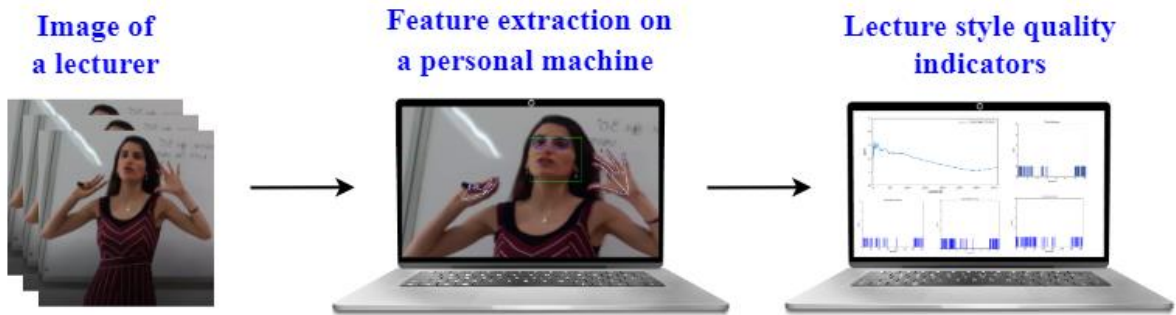
Figure 4.1 : Automated TSA tool. A video of a lecture captured by an ordinary camera is analysed to extract lecture style quality indicators.
