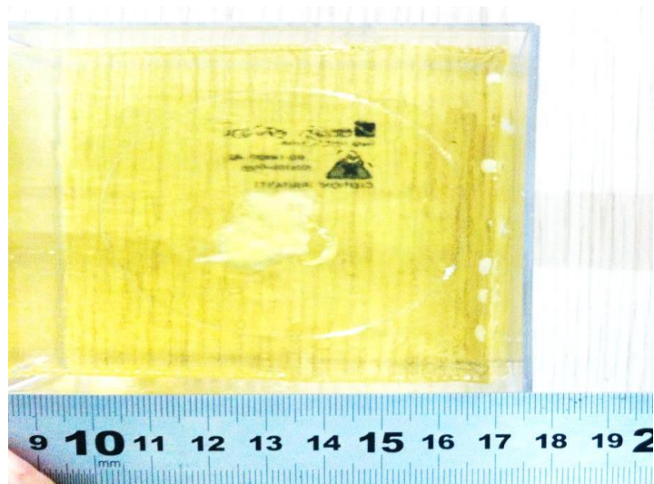
Figure 7.5: Thermal lesions in a commercial polyacrylamide gel with acoustical power 10 W for 5 s from the top.
