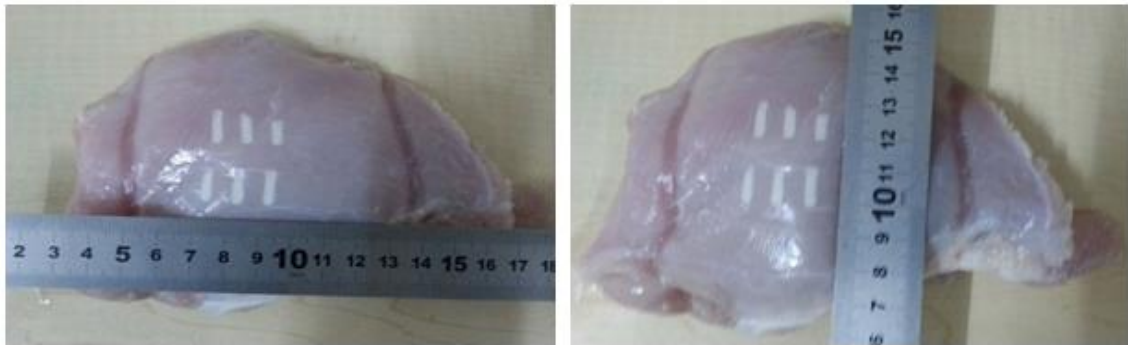
Figure 7. 2: Thermal lesions in a freshly turkey tissue phantom with acoustical power 20 W for 10 s.
