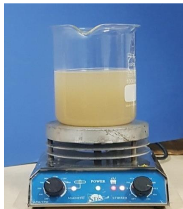
Figure 4.2: The preparation of the atherosclerotic plaque phantoms using the magnetic stirrer.
