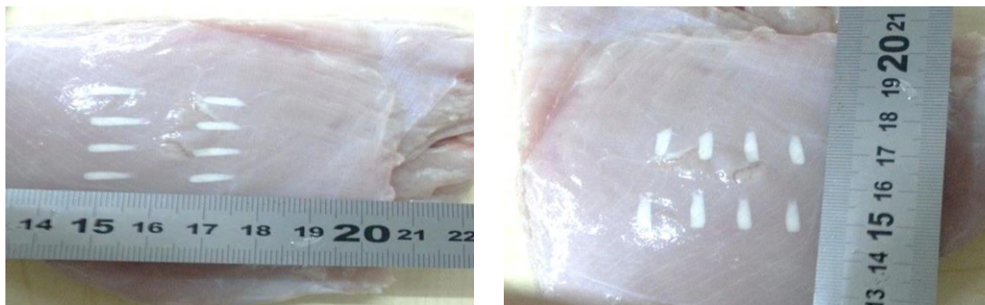
Figure 7. 2: Thermal lesions in freshly turkey tissue phantom with acoustical power 13 W for 10 s.
