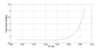
Figure 10: Effect of TIT on total operation cost ( $r_{cT} = 13.5$ ,  $r_{cB} = 4$ , optimum MFRR)
