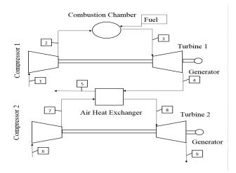
Figure 1: ABC without intercooling integration in the bottoming cycle
