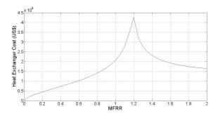
Figure 6: Effect of MFRR ratio on air heat exchanger cost ( $r_{cT} = 14$ ,  $r_{cB} = 4$ , TIT=1500 K)
