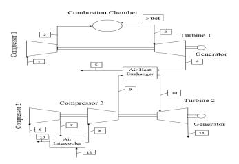
Figure 2: ABC with intercooling integration in the bottoming cycle
