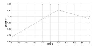
Figure 4: Effect of MFRR ratio on efficiency ( $r_{cT}$ =14,  $r_{cB}$ =4, TIT=1500 K)
