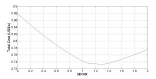
Figure 5: Effect of MFRR ratio on total operation cost ( $r_{cT} = 14$ ,  $r_{cB} = 4$ , TIT=1500 K)
