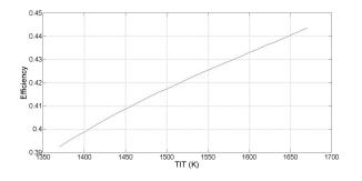
Figure 9: Effect of TIT on overall efficiency ( $r_{cT} = 13.5$ ,  $r_{cB} = 4$ , optimum MFRR)
