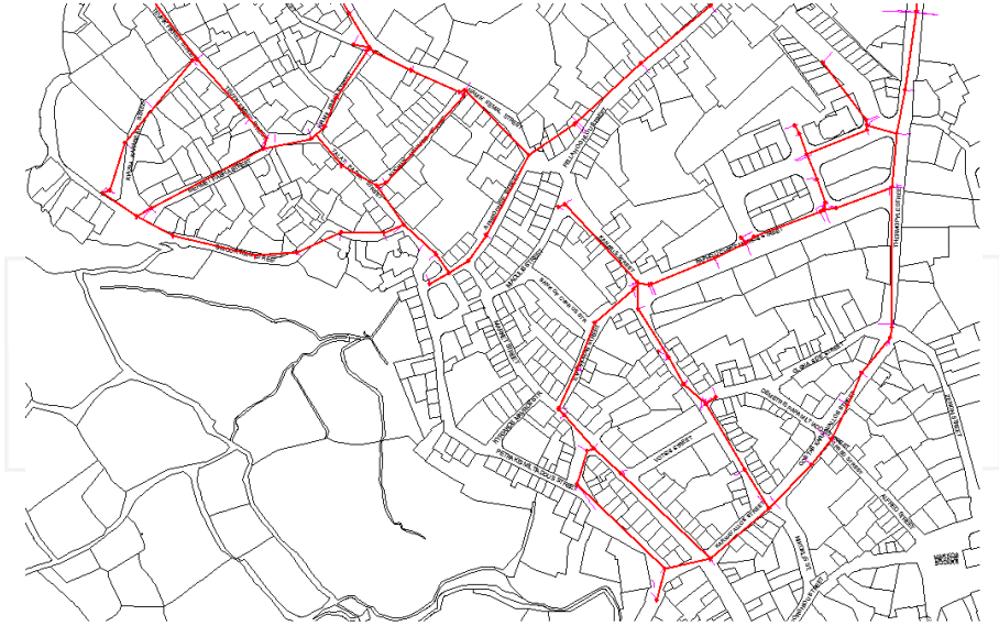
Figure 4. The water network following the GPR survey
