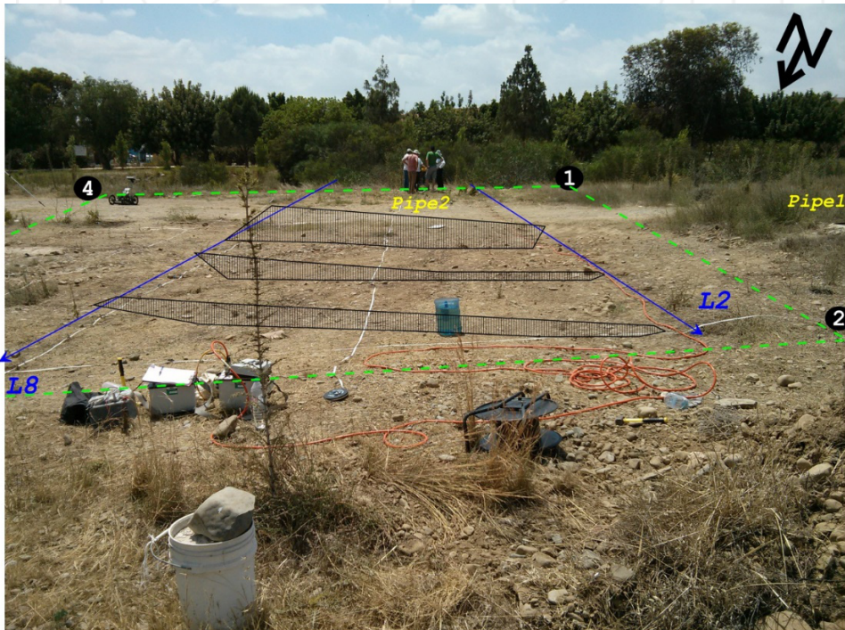
Figure 8. Outline of the footprint of water flow on the ground surface based on the results of the ERT monitoring experiment.
