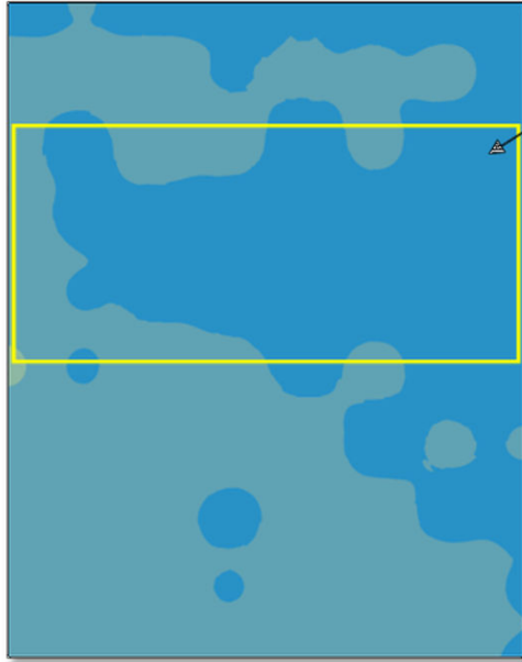
Figure 6. Ground temperature over the area of interest as recorded from the digital laser thermometer, before the leakage event. Rectangle indicates the location of the buried pipeline. Blue values indicates temperatures 14-16°C while the cyan colour temperatures 16-18°C.
