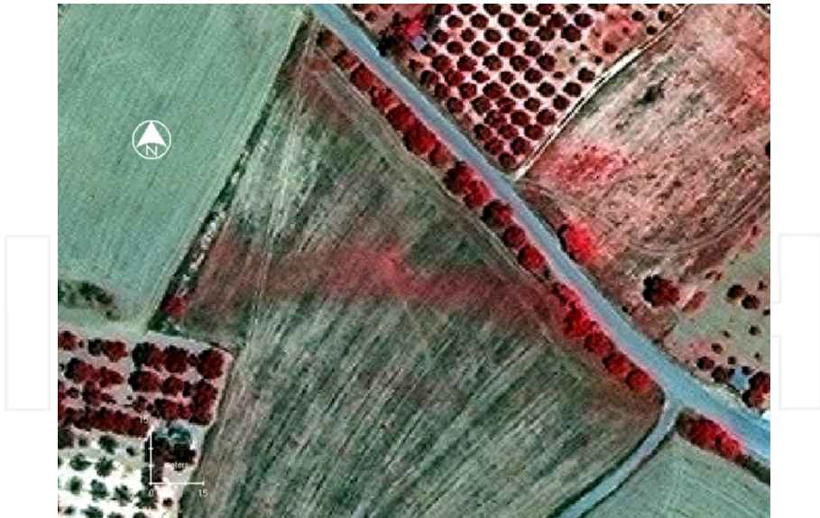
Figure 27. Detection of leakage problem using high resolution satellite data (Agapiou et al. 2014)
