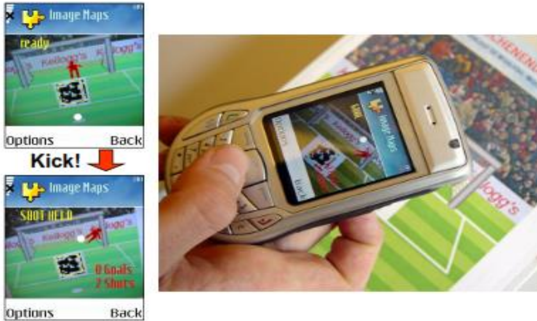
Figure 2.4: “Penalty Kick” (Rohs, 2007), the screen shows a virtual goalkeeper inside the field image which is used as a marker and the user aims by rotating and tilting the phone.
