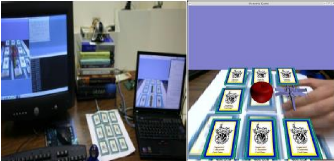
Figure 2.7: Memory AR (Diaz et al., 2006), game setup with the real board of cards (left), the augmented environment of the board (right)
