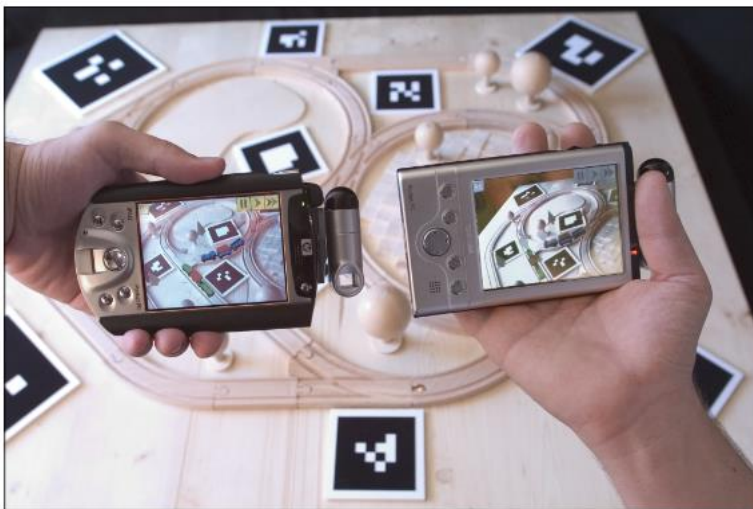
Figure 2.5: “The Invisible Train” (Wagner, Pintaric, Ledermann, & Schmalstieg, 2005), the user can interact with specific virtual trains and rail switches only when points the device at the railway and markers around it.
