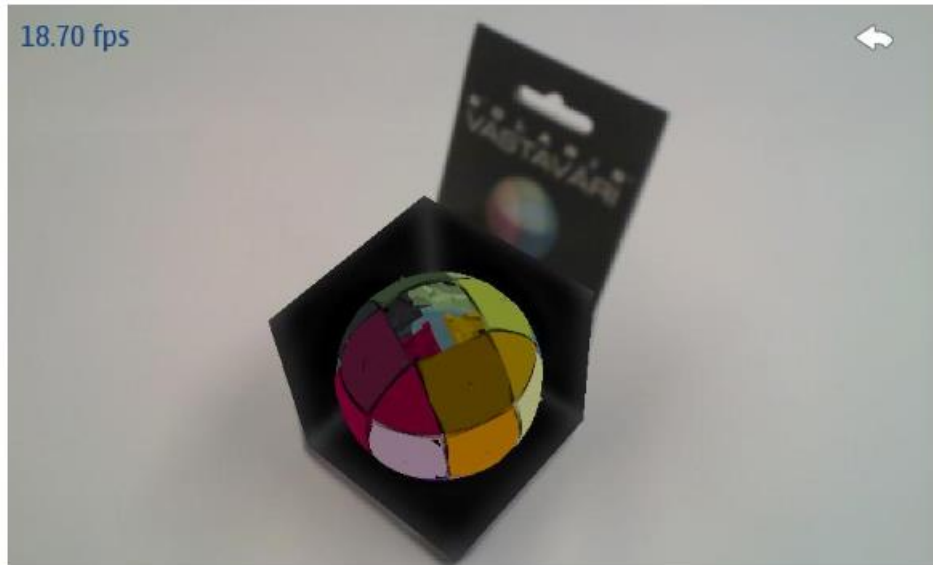
Figure 2.2: A virtual 3D object is augmented on top of the package to allow users see how the inside product looks like (Välkkynen et al., 2011)
