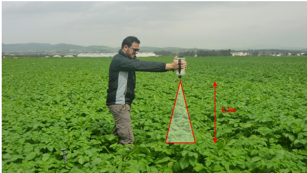
Figure 3.8. Field spectroradiometric measurements acquired over potatoes in Mandria village, Paphos, Cyprus
