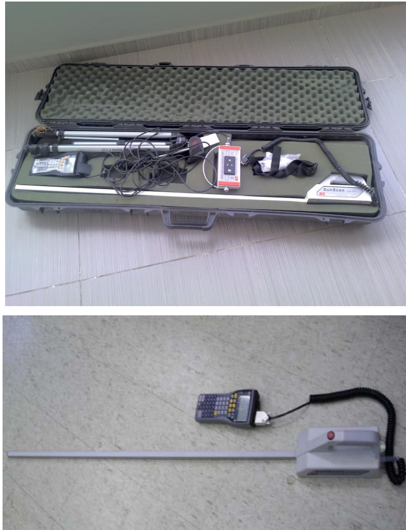
Figure 2.5. SunScan (Delta-T) canopy analyser for LAI and crop height measurements
