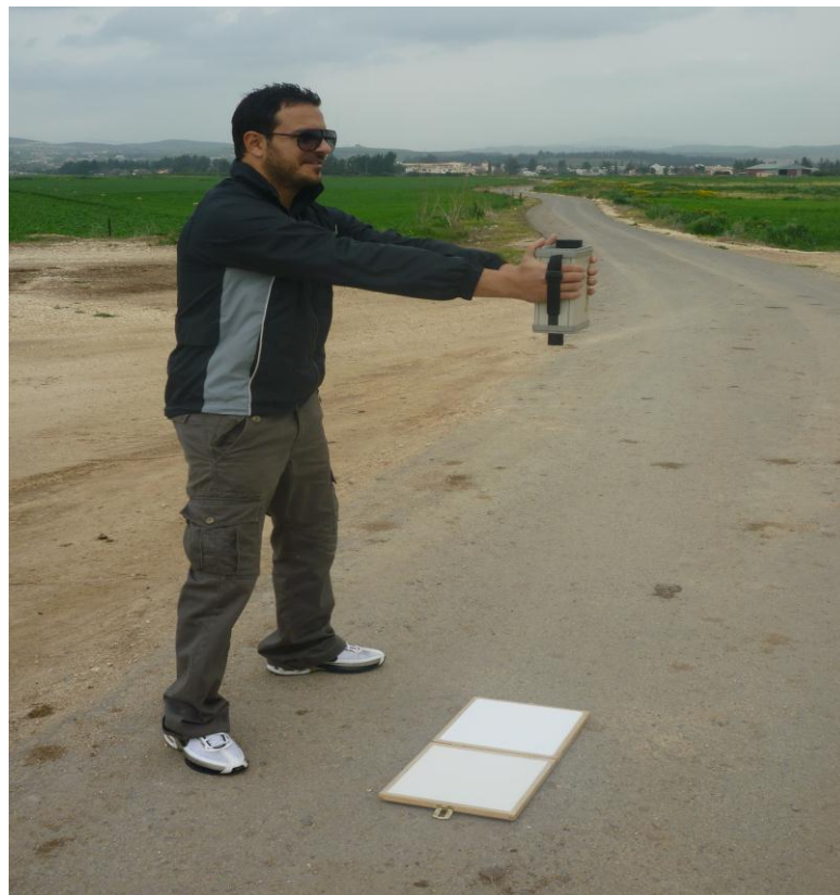
Figure 2.4. Technique of using spectroradiometer and spectralon
