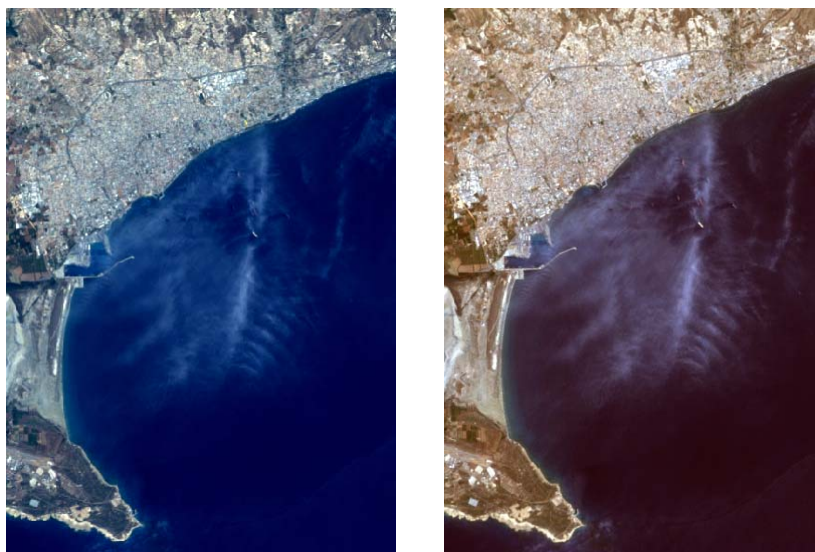
Figure 8-20 Satellite images acquired 16/6/2010, before (left) and after (right) atmospheric correction using DP method
