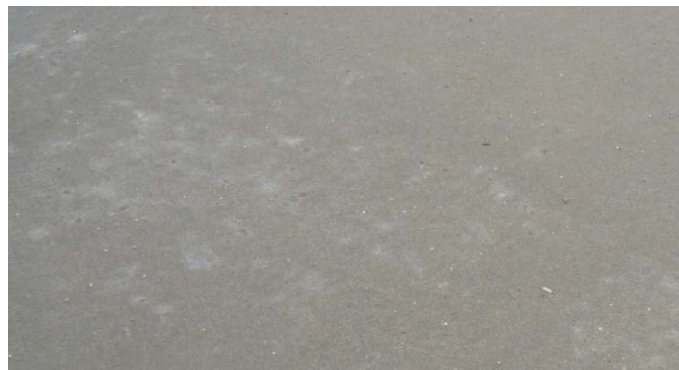
Figure 7-19 Salinization of Compacted Sand
