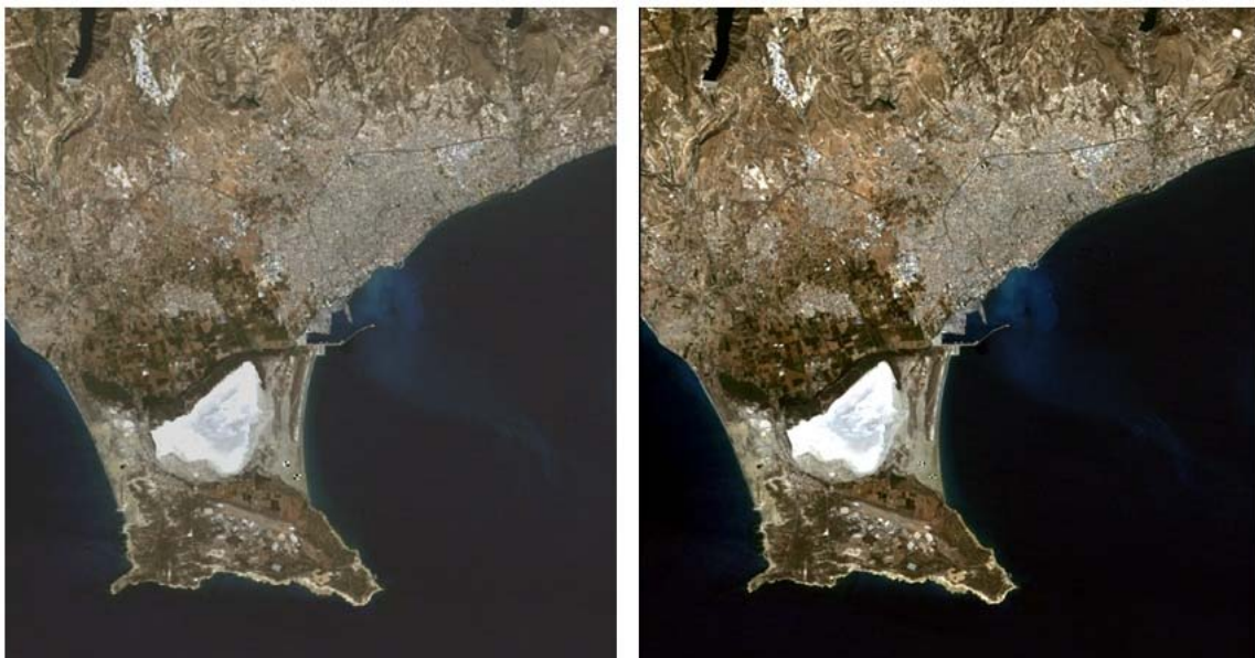
Figure 8-26 Satellite images acquired 27/8/2010 before (left) and after (right) atmospheric correction using DP method
