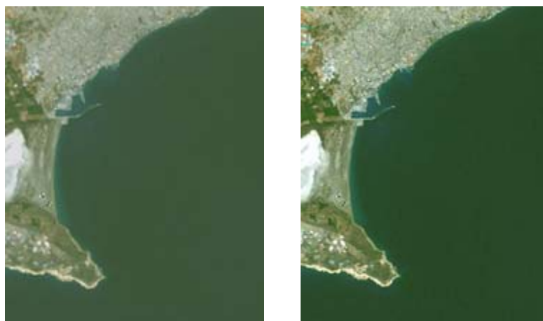
Figure 8-32 Satellite images acquired 9/12/2010 before (left) and after (right) atmospheric correction using DP method
