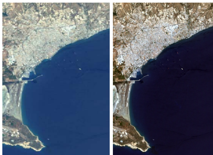
Figure 8-18 Satellite images acquired 31/5/2010 before (left) and after (right) atmospheric correction using DP method
