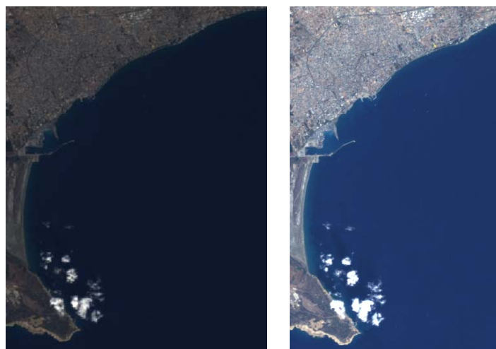
Figure 8-30 Satellite images acquired 7/11/2010 before (left) and after (right) atmospheric correction using DP method
