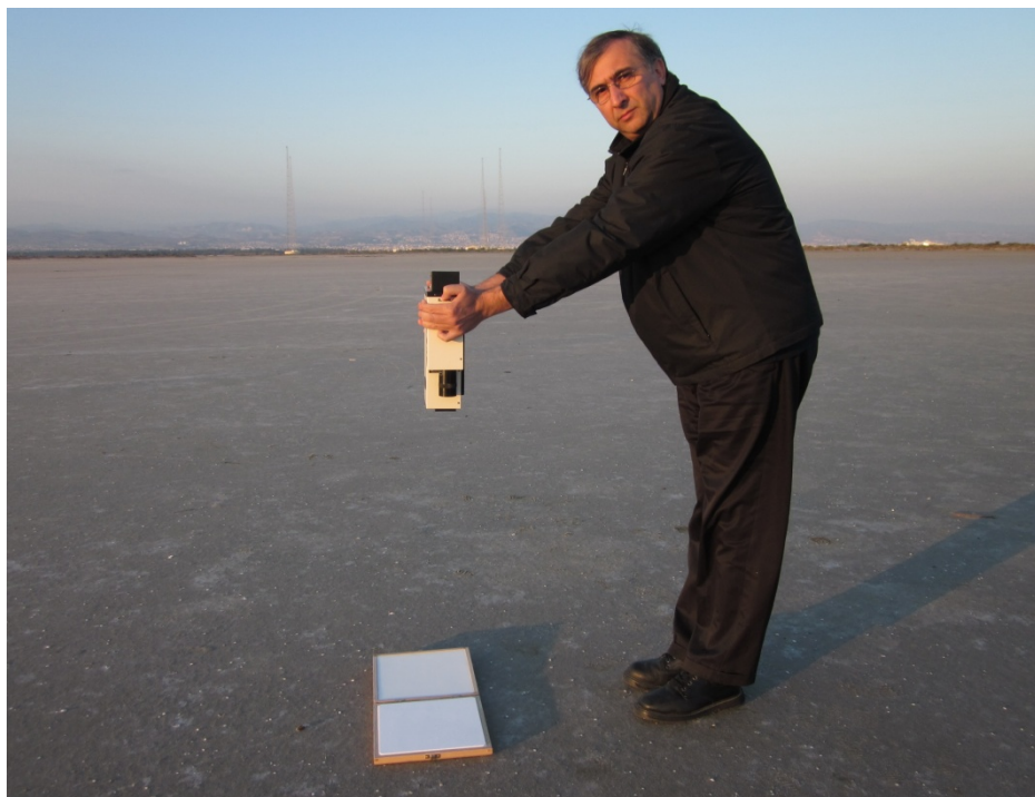
Figure 5-1 Field spectroradiometric measurement using a white spectral panel at the Compacted Sand target
