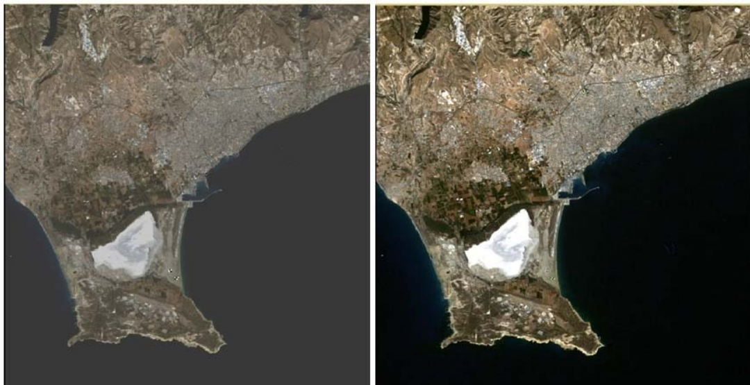
Figure 8-28 Satellite images acquired 28/9/2010 before (left) and after (right) atmospheric correction using DP method
