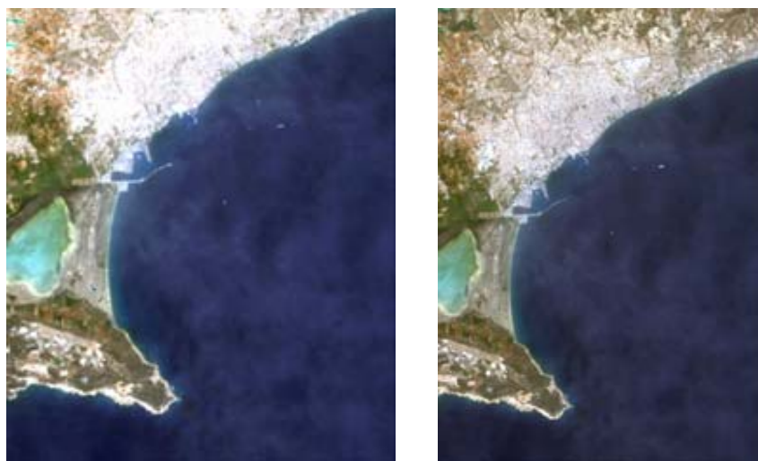
Figure 8-34 Satellite images acquired 2/5/11 before (left) and after (right) atmospheric correction using DP method
