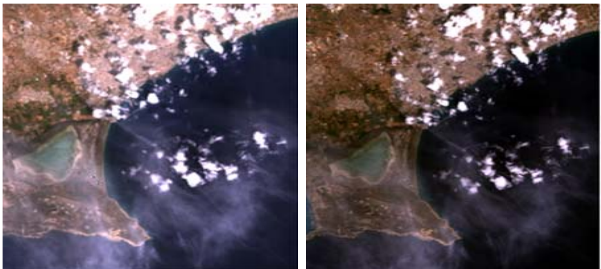
Figure 8-16 Satellite images acquired 29/4/2010 before (left) and after (right) atmospheric correction using DP method
