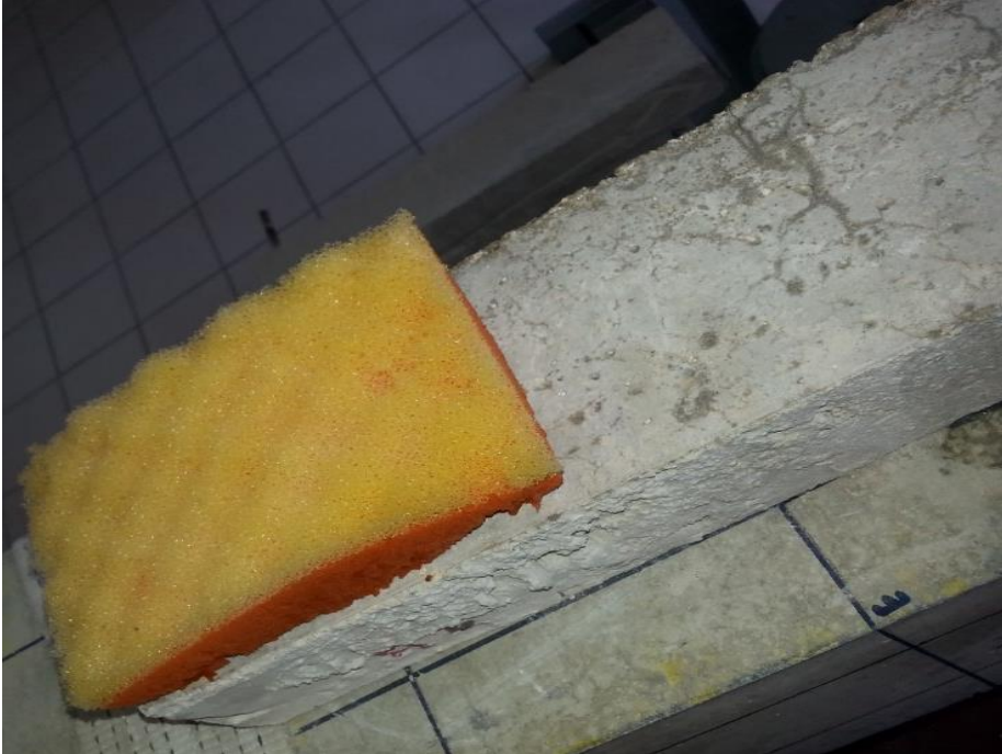
Figure 14: Wetting of the specimen surface using a sponge
