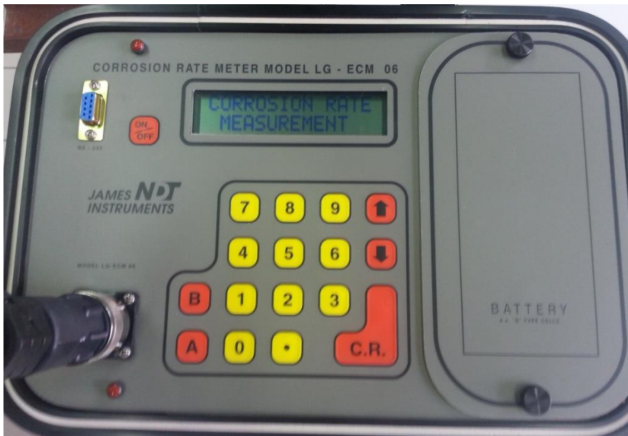
Figure 11: GECOR6 Corrosion Rate Meter apparatus
