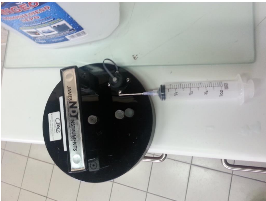
Figure 12: Filling the A sensor with solution liquid
