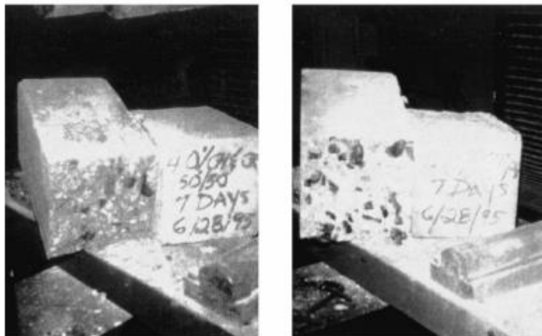
(b) Distribution of Crumb and Chip Particles in the Rubberized PCC Mixtures
