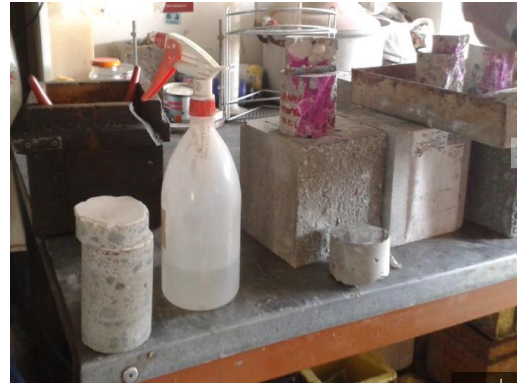
Figure 23: The sample after its contact with phenolphthalein
