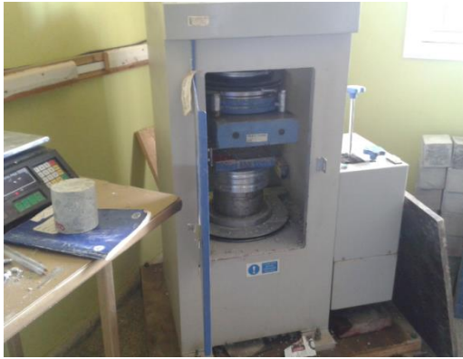
Figure 24: Device which exert pressure on each sample until it break
