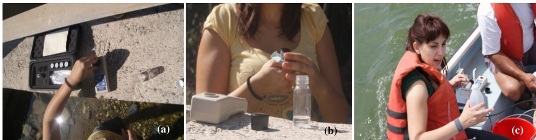
Figure 3. 20: (a-c) The portable Palintest Micro 950 Waterproof used to determine the turbidity level at several water samples during in situ campaigns.
