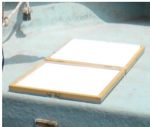
Figure 3. 16: Standard spectralon panel (Lambertian surface) used as reference value for the downwelling irradiance.
