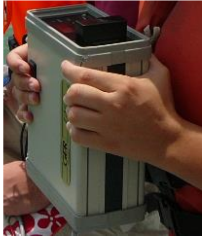
Figure 3. 17: Handheld field spectroradiometer GER1500 covering the UV-Vis-NIR area of the spectrum.
