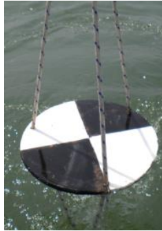
Figure 3. 19: A Secchi Disk used during the field campaigns to measure the Secchi Disk Depth.
