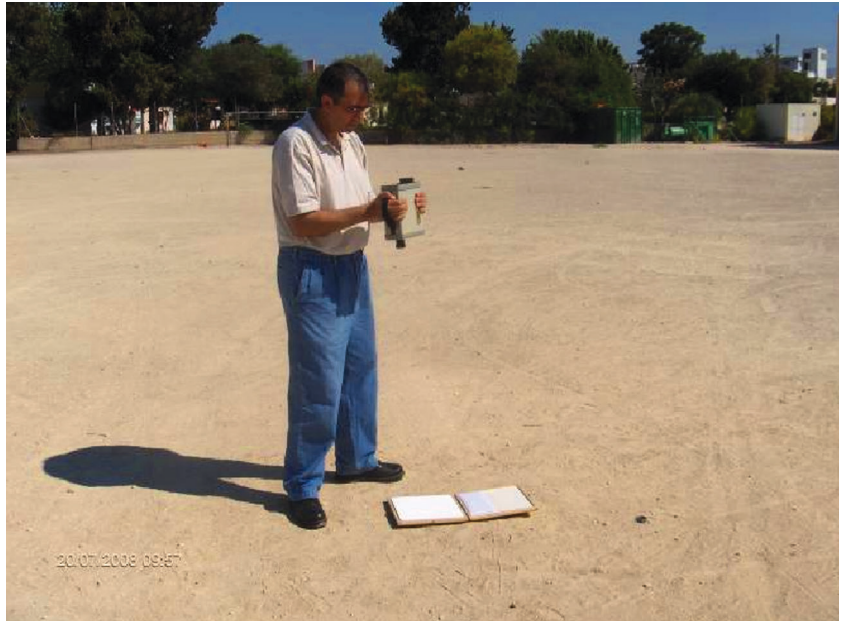
Figure 15: In situ spectroradiometric observations using the GER1500 field spectro-radiometer.
