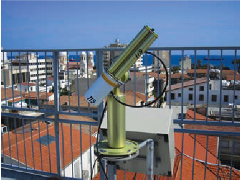
Figure 6: CIMEL SUN-PHOTOMETER (Cyprus University of Technology Premises-Remote Sensing Lab)
