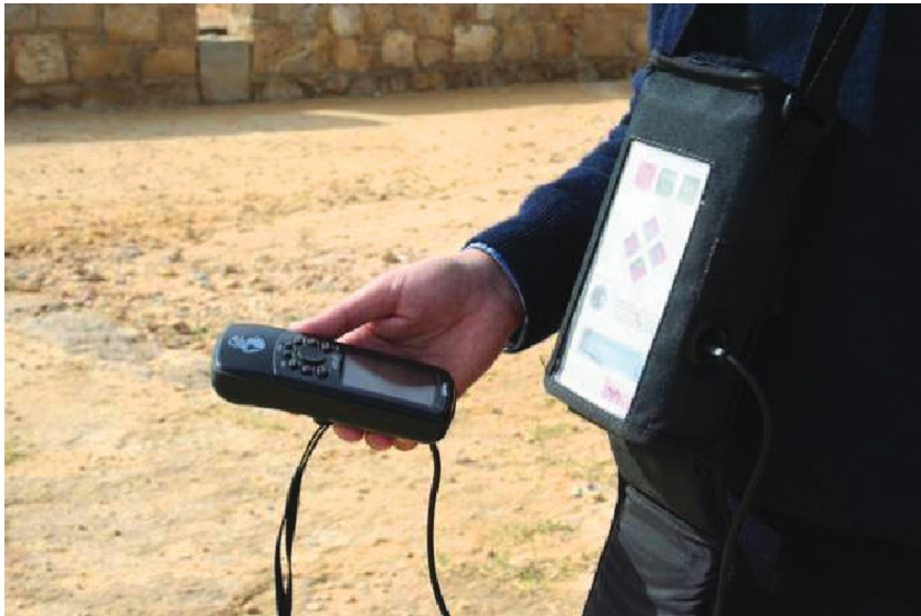
Figure 7: Hand-held Sun photometer - Microtops II (Cyprus University of Technology Premises-Remote Sensing Lab)
