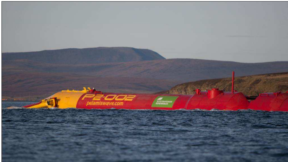
FIGURE 1. Pelamis Wave Power Device, picture from http://www.pelamiswave.com
