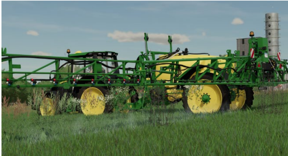
Figure 3: Variable rate weed control with a camera and individual nozzle control
