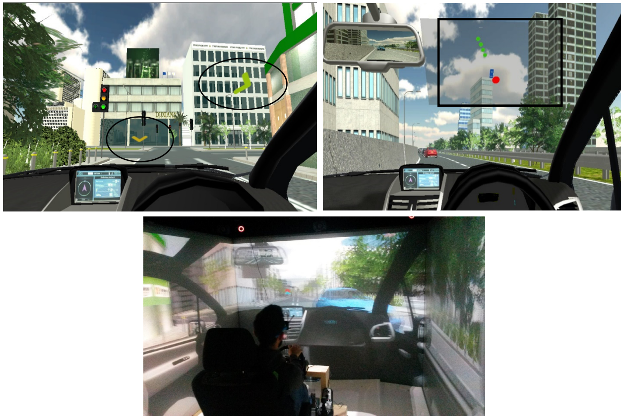
Figure A2. Screenshot from the first-person view of the Arrows (top left) and Radar (top right) designs on the HUD. Superimposed icons on the HUD show visualisations of TSRs. Arrows show imminent vehicle threats about to emerge at intersection (right arrow) and a vehicle following closely (lower-centre arrow). Radar shows host vehicle as a blue car in the centre of radar and traffic hazards as red circles. Below a participant engaging a scenario during an experiment in VR cave simulator using the Radar design.
