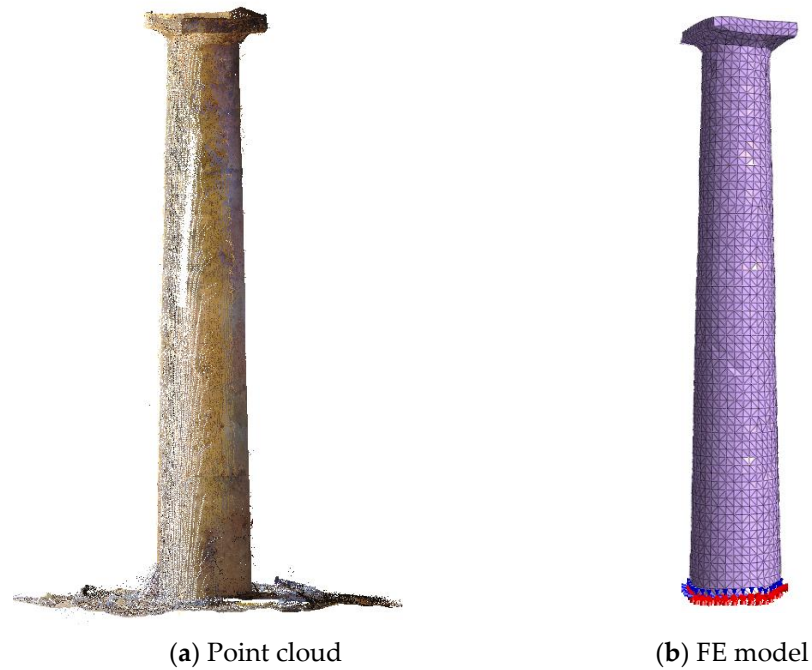
Figure 6. Example of the conversion of a point cloud (a) into FE model (b). This example shows one of the columns of Tombs 7 in Tombs of the Kings in Paphos, Cyprus.
