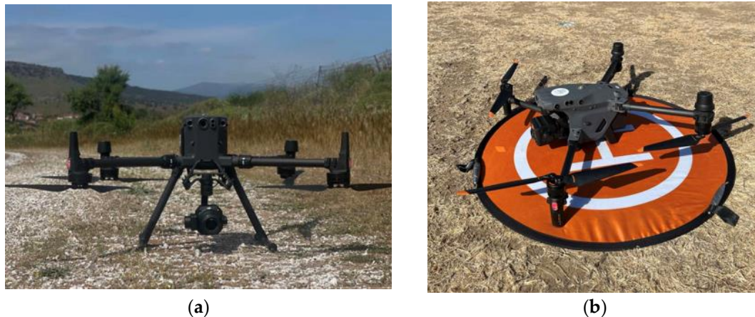
Figure 2. Equipment for the implementation of the ALTITUDE platform: (a) DJIMatrice M30T, DJI, Shenzhen, China, used for mapping with the DJI P1 camera and inspections with the DJI H20T camera; (b) DJIMatrice M300, DJI, Shenzhen, China, used for inspection of the power transmission network.
