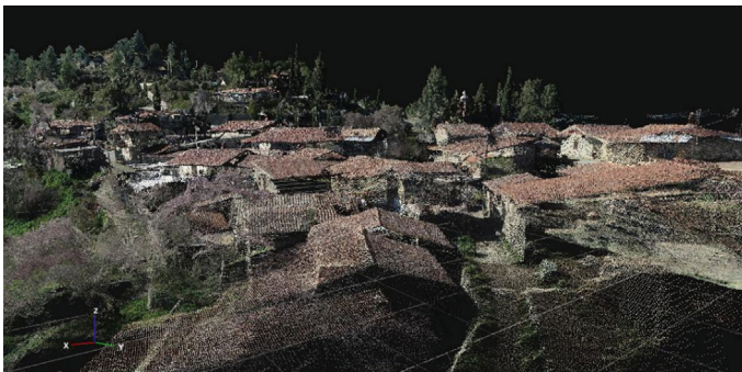
Fig. 5 3D dense point cloud from drone photogrammetry © UNESCO chair on digital cultural heritage
