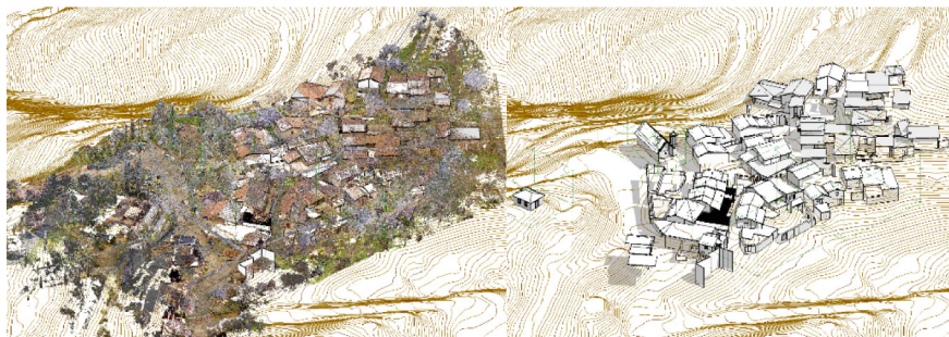
Fig. 6 Creation of the BIM model using as base the point cloud of terrestrial laser scanner and drone © UNESCO chair on digital cultural heritage
