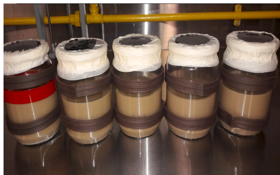
Fig. 2. Bentonite preparation for (a) dry and (b) wet/thermal activation methods.
