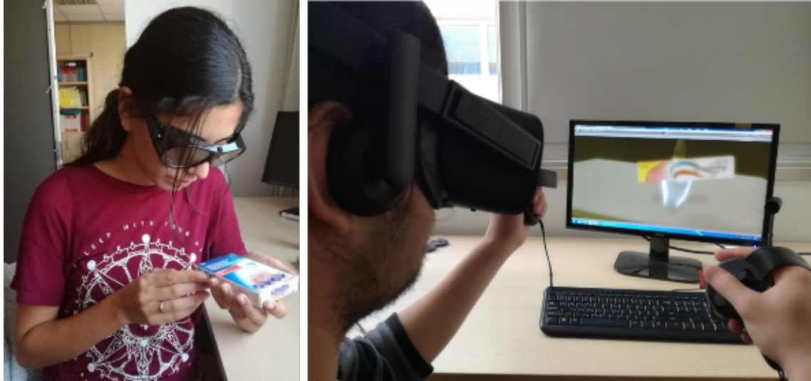
Figure 5.17 Evaluation of product packaging design using the simulation goggles (left) and the VR-based simulation (right).
