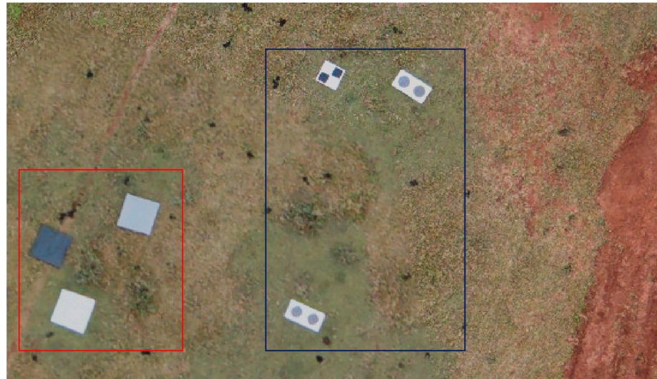
Figure 5. Targets located near the overflow area. The radiometric targets are in red, and the GCPs are in blue.
