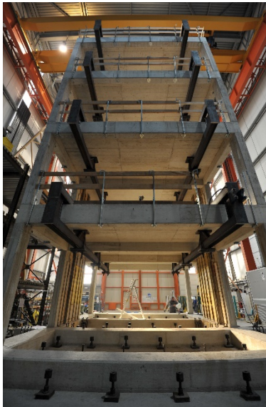
Figure 5.4 Actuator attachment beams
