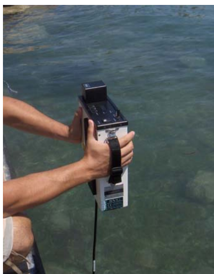
Figure 2. In-situ spectroradiometric measurements using the GER1500 field spectroradiometer and fibre-optic probe (13/8/2008, Paphos)
