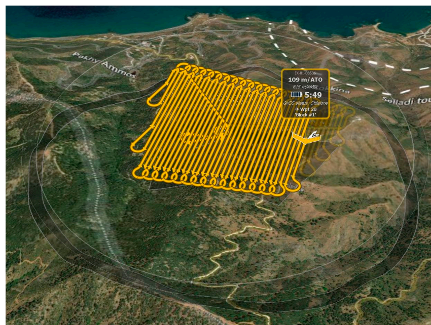
Figure 5. Flight Planning using the eMotion Software.
