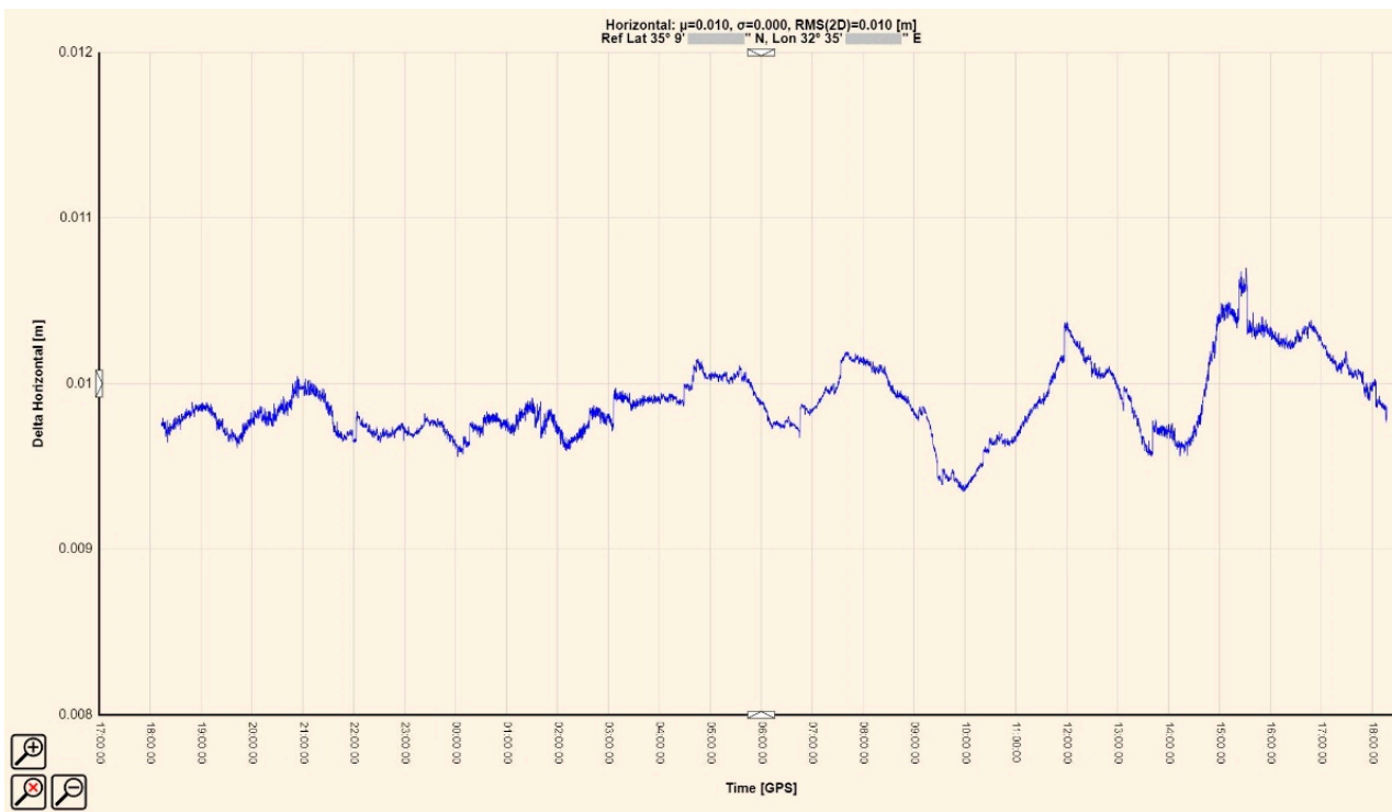
Figure 23. The horizontal stability of the ALEV GNSS monument in 24 h observations.
