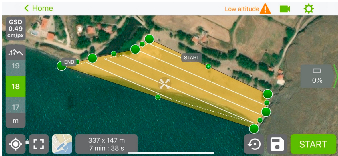
Figure 3. Pix4D capture of UAS mission planning preview for Xabelia beach.
