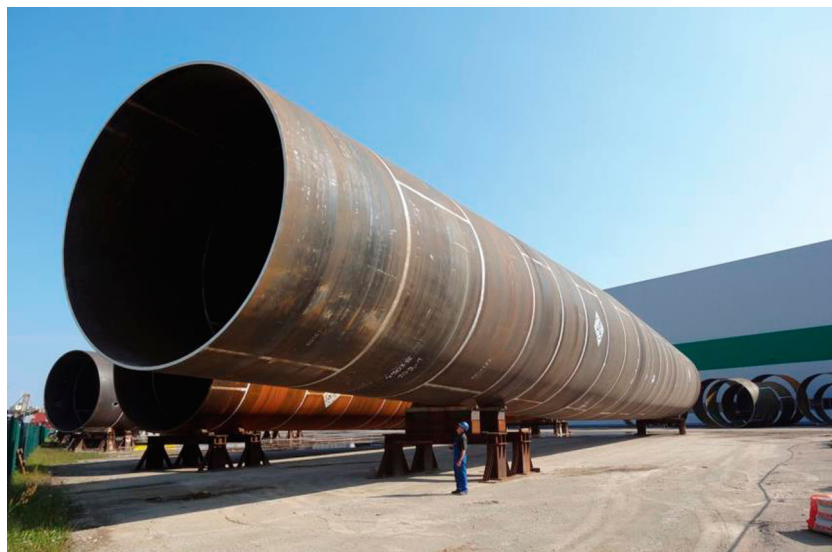
Figure 2. A fabricated monopile for an offshore wind farm (Kallehave et al. 2015) (This figure is available in colour online).
