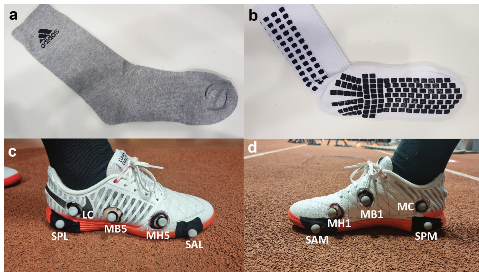
Figure 1. The regular sock (a), the grip sock (b), the indoor football shoe (c and d) with markers attached to the shoe midsole: posterior lateral (spl), anterior lateral (sal), anterior medial (sam), posterior medial (spm). Foot marker locations: first metatarsal head (mh1), first metatarsal base (mb1), fifth metatarsal head (mh5), fifth metatarsal base (mb5), lateral calcaneus (lc), and medial calcaneus (mc).
