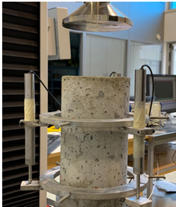
Figure 2. Cyclic compressive loading specimen setup.
