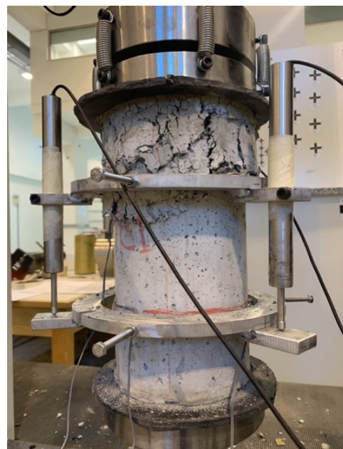
Figure 9. Cyclic Compressive Loading Specimen B1 at 20 mm Displacement.
