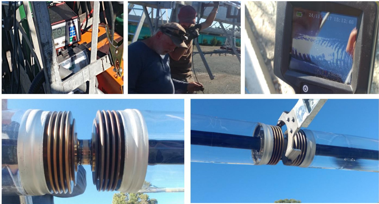
Figure 86: Testing the welding by a camera.
