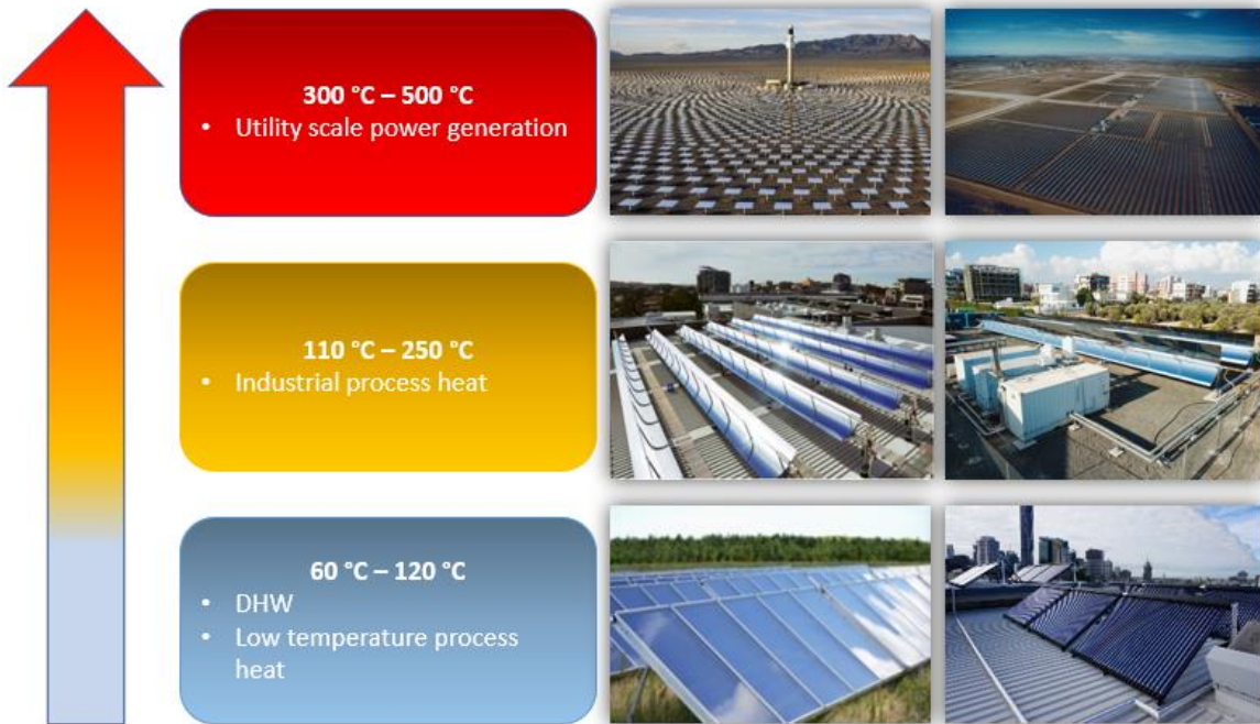
Figure 1: Technology choice depends on application temperature.
