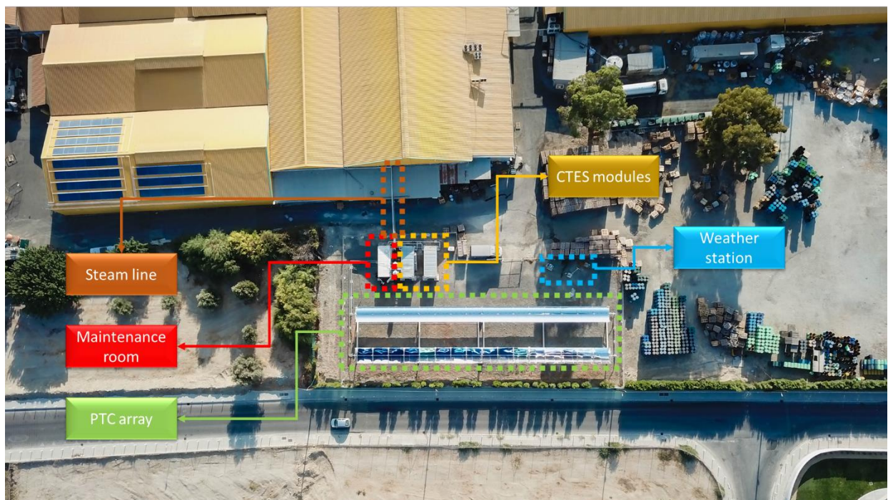
Figure 43: Sky-view showing the KEAN factory and the location of the PTC system and its components.
