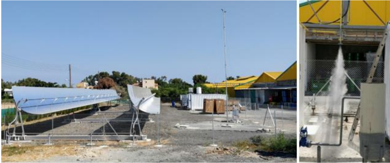
Figure 99: First operation tests and steam production @10 bar pressure.
