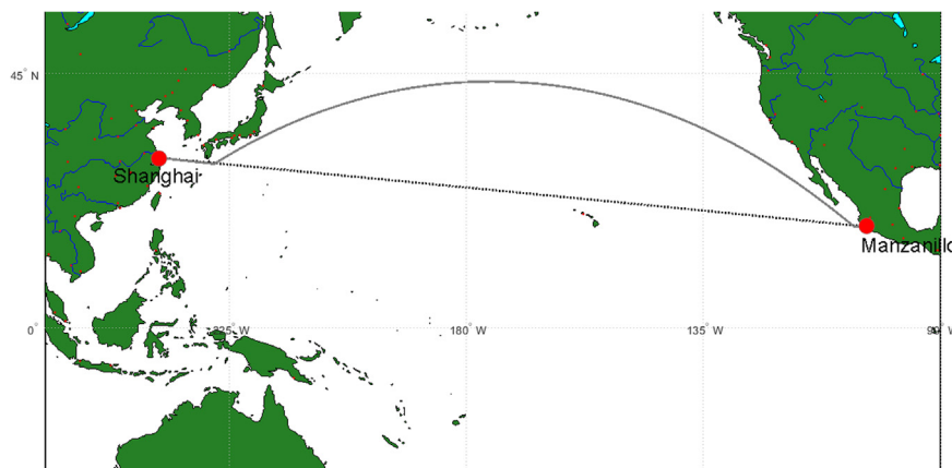
Fig. 5. Great circle (solid) and rhumbline (dashed) route for the Pacific Ocean crossing.
