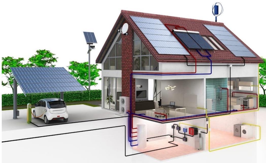
Figure 1.1: Typical example of a nZEB building
