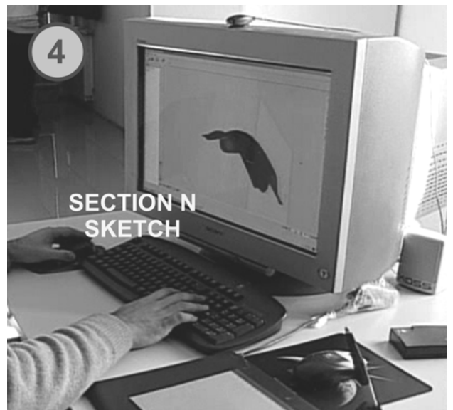
Fig. 9. Shape modelling: 1 – 6DOF sketch plane; 2 – Sketch plane positioning and orientation in the 3D space; 3 – First and 2 nd section curve are joined together; 4 – N section curves are joined to create the final NURBS surface.
