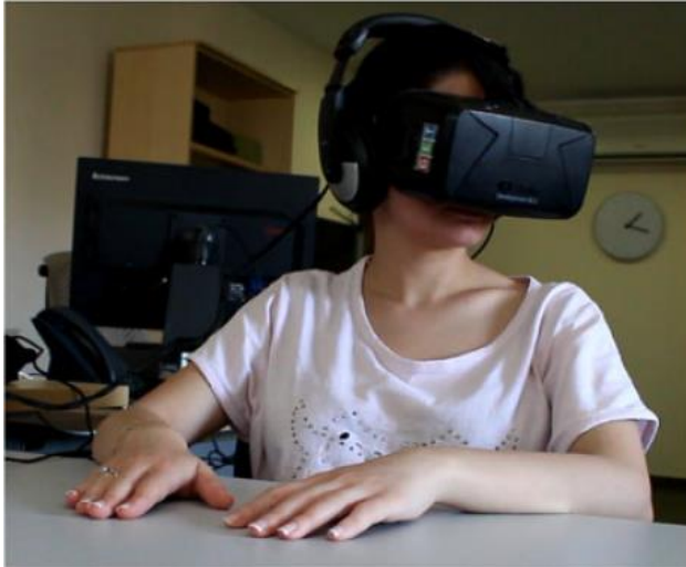
Figure 4: Participants in Experiment 1 were fitted with an HMD for stereo display and head tracking, and headphones for stereo sound
