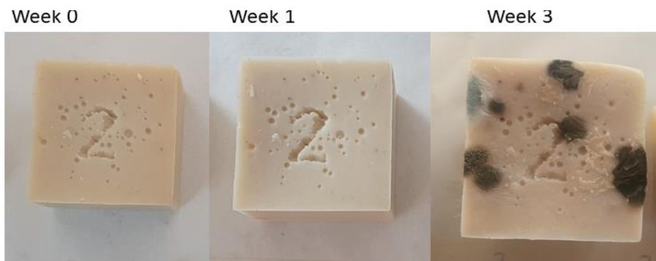
Figure 48 : Sample 2; progress from week 0 to week 3 (containing 30 % evaporated milk and 0.4 % sodium benzoate, stored at 4°C)
