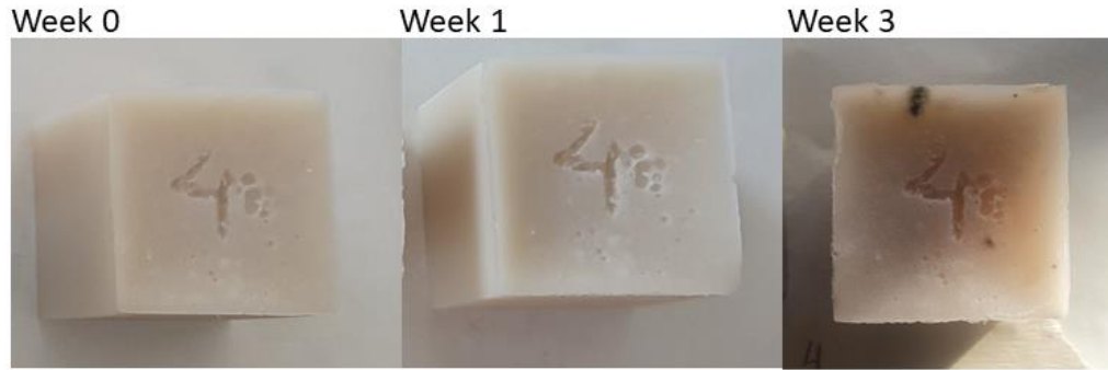
Figure 50 : Sample 4; progress from week 0 to week 3 (containing 0 % evaporated milk and 0.4 % sodium benzoate, stored at 4°C)
