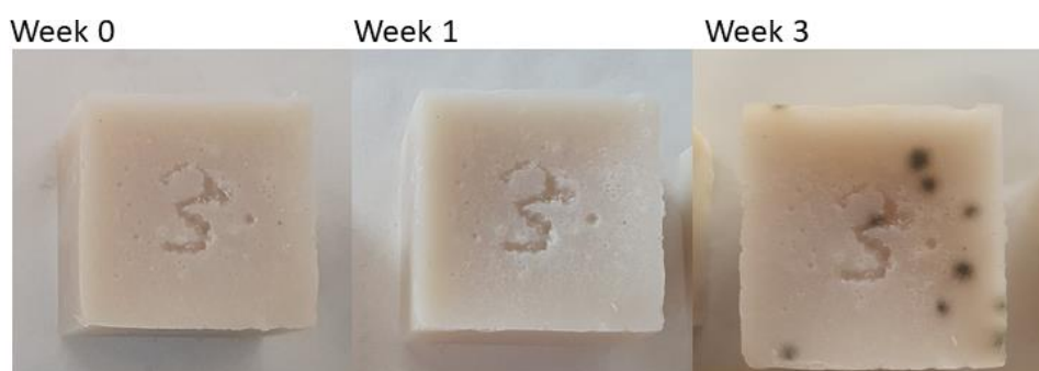
Figure 49 : Sample 3; progress from week 0 to week 3 (containing 0 % evaporated milk and 0 % sodium benzoate, stored at 4°C)
