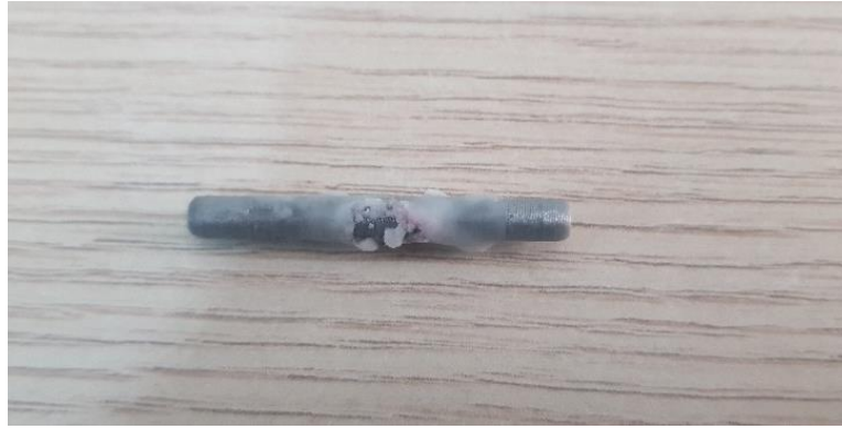
Figure 11 : The disrupted layer of wax on the tube caused by the ultrasound sonication.
