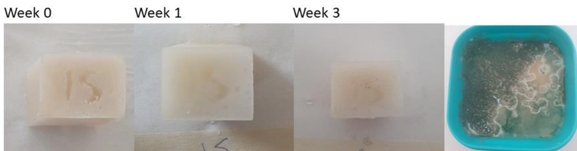
Figure 59 : Sample 15; progress from week 0 to week 3 (containing 0 % evaporated milk and 0 % sodium benzoate, stored in glycerol/water at 25°C)
