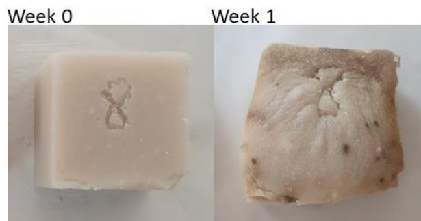
Figure 54 : Sample 8; progress from week 0 to week 3 (containing 0 % evaporated milk and 0.4 % sodium benzoate, stored at 25°C)
