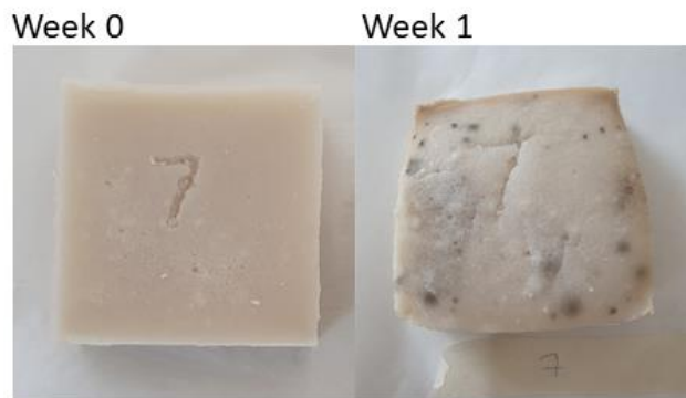
Figure 53 : Sample 7; progress from week 0 to week 3 (containing 0 % evaporated milk and 0 % sodium benzoate, stored at 25°C)
