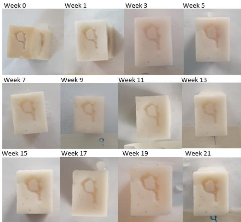
Figure 55 : Sample 9; progress from week 0 to week 21 (containing 30 % evaporated milk and 0 % sodium benzoate, stored in glycerol/water at 4°C)
