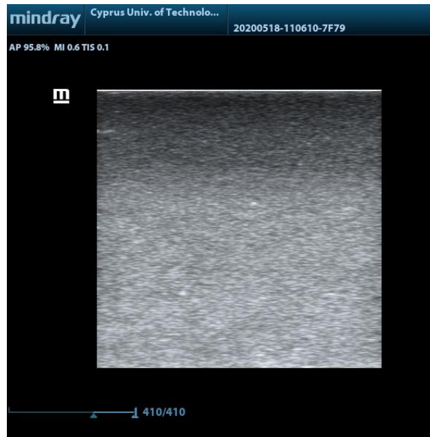
Figure 30 : Ultrasound image of the sample with the optimum recipe (6 % agar, 4 % silicon dioxide).
